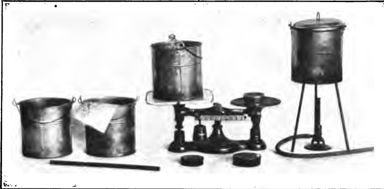
FIG. 20. Apparatus used to show that equal weights of ice and ice water have different cooling effects.
